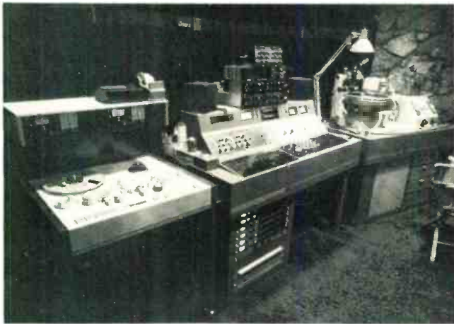
Woodland's disc mastering facility—equipped with Neumann's SAL 74 cutting system.
