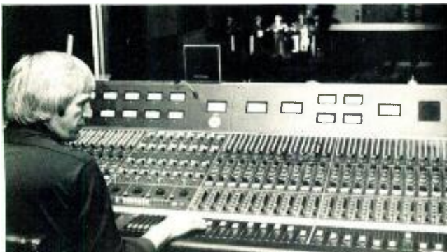
The Neve 40-input custom mixing console used in the broadcast of the Grand Ole Opry over WSM Radio.
