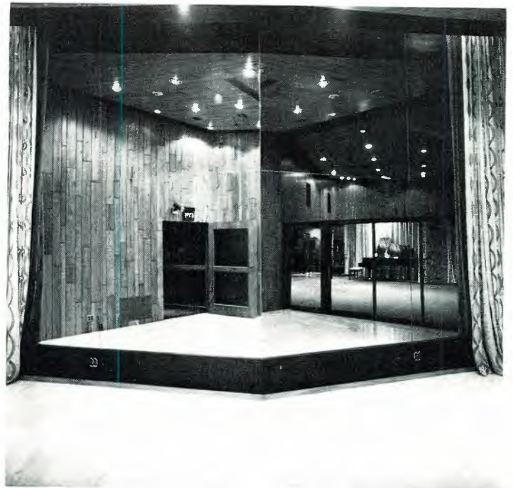
Angled mirrors forming walls of Studio D string room enhance acoustics and provide important sight lines to other areas of the studio.
