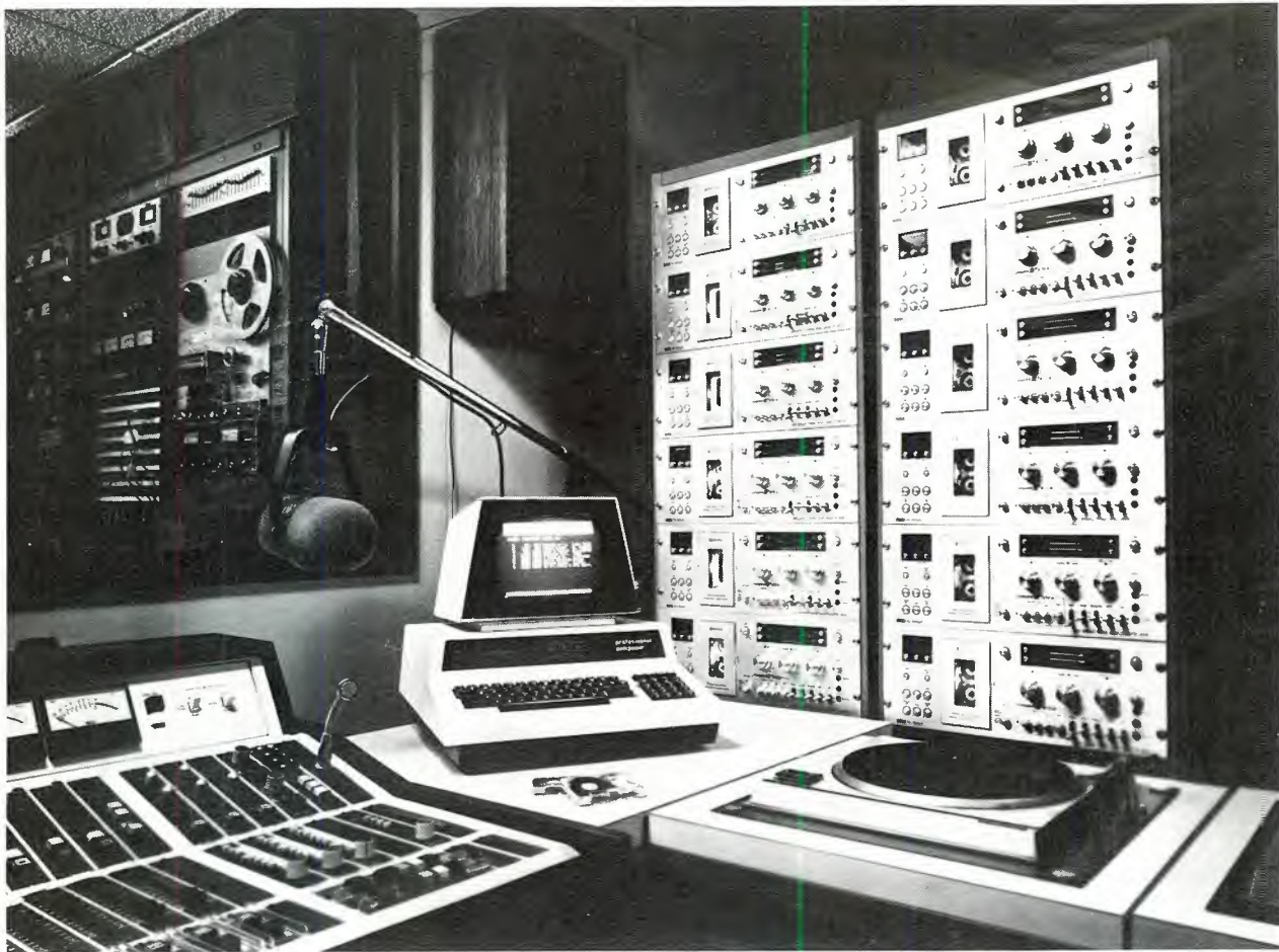
In the foreground, a Commodore PET micro-computer handles programming chores, keeping track of ten or more cassette decks.
