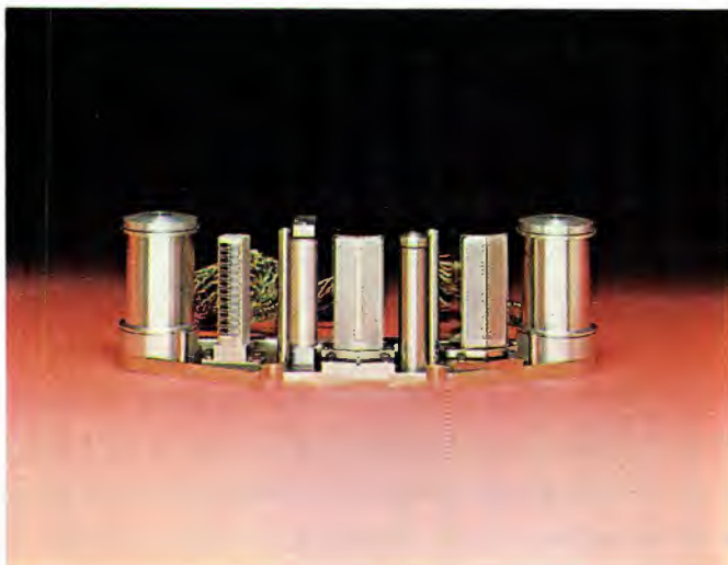
Figure 3. The tape guides on either side of the heads are an integral part of the head block assembly, thus minimizing tape path alignment problems when changing between 16- and 24-track head stacks.
