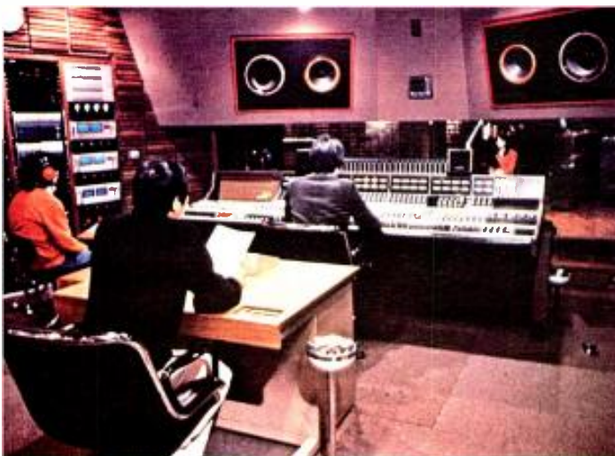
Figure 5. Studio 3 control room. Each control room has a 32 in/24 out Automated Processes console. The 16- and 24-channel recorders are Studer A-800s, and the 2-channel machines are Studer A-80s and Ampex ATR-100s.
