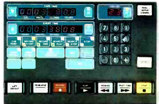
ATR-124's Multi-Point Search-To-Cue (MPSTC). Provides 100 cue locations.
