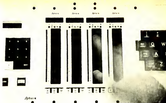
Figure 3. The fader computer recognizes only finger movement, and not where it is positioned in the infra-red field.
