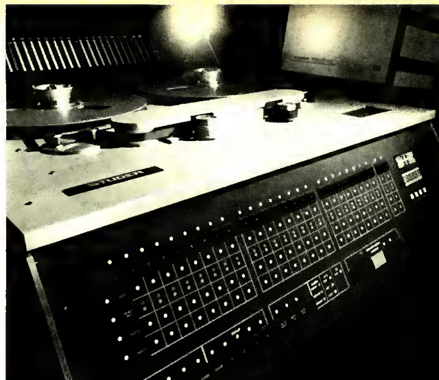
Figure 3. Studer's entry in the digital arena: 24 audio tracks on half-inch tape at 30 ips.
