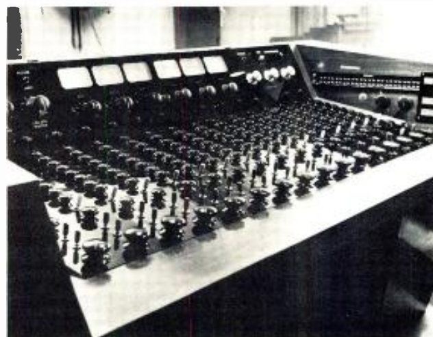
Criteria's first state-of-the-art console in 1957, a 3-track tube console.
