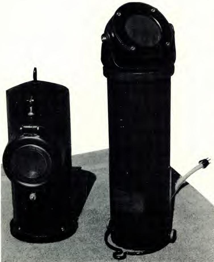
Figure 6. Condenser microphones, circa 1928. A General Electric microphone built for RCA and the Westinghouse model 47A.
