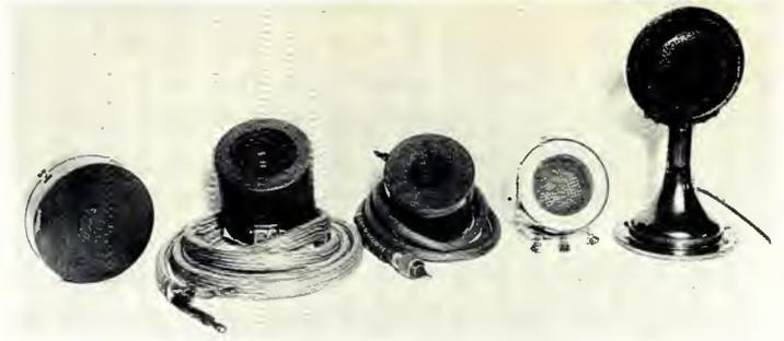
Figure 5. A collection of early Westinghouse microphones. From left to right: glow discharge, push-pull condenser, standard condenser, double-button "tomato can," and a double-button carbon mic in a special desk stand.
