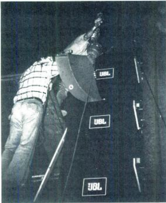
Installing the woofers in their enclosures, backstage before mounting in speaker clusters. Note the use of fiberglass for damping of spurious resonances.
