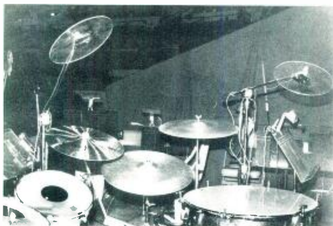
The microphone set-up, employing several PZM mics mounted on plexiglass disks, for the Ringling Bros. orchestra.
