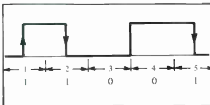
Figure 4. An example of MFM (Modified Frequency Modulation) encoding.
