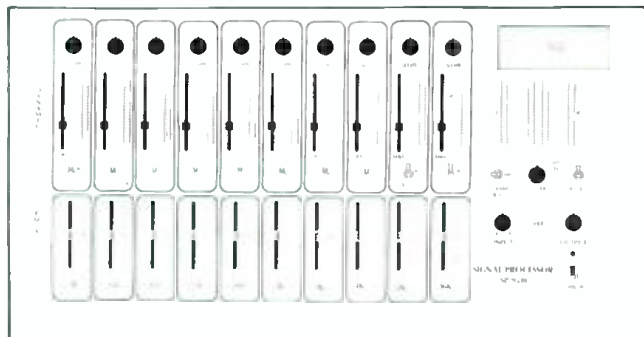
Figure 4. The front panel layout for Broadcast Technology's SP 9511 ten-band signal processor.
