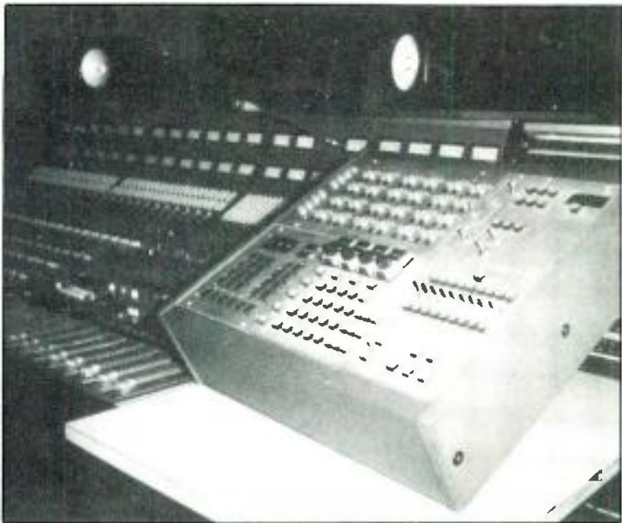
Bearsville's "Assistant's panel," named because of its location on the assistant's desk to the right of the console
