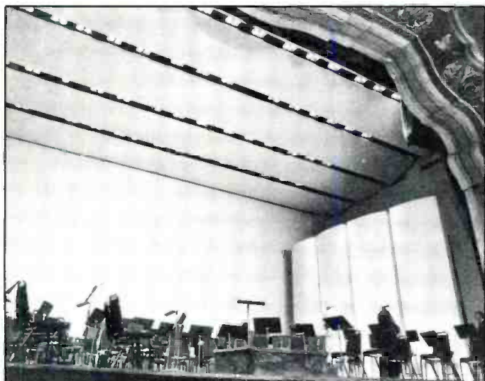
Figure 4. The mechanized stage enclosure in the symphony orchestra configuration.
