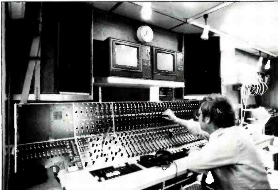
Figure 7. Control room of a mobile studio featuring a 30-channel Glen Sound mixing desk and Studer B62 recorders.
