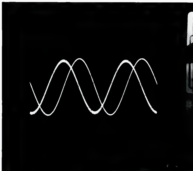
Figures 6A and 6B. Input and surround channel output signals are compared with time delay set to minimum (A) and to maximum (B).
