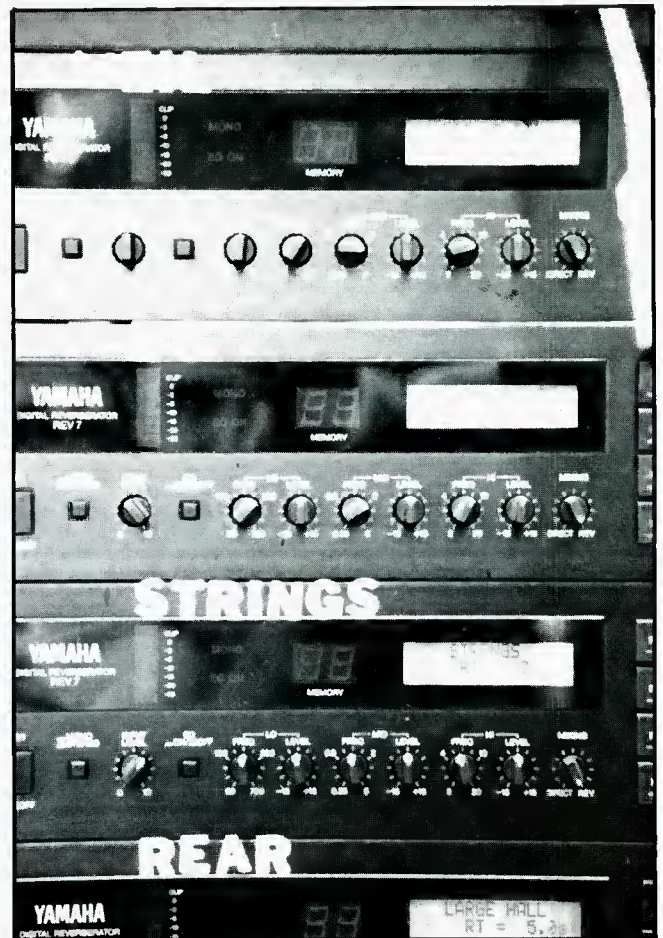
These Yamaha REV-7 units are part of the signal processing system.
