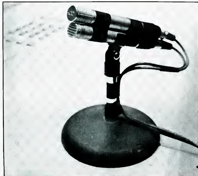
Figure 10. As one possible arrangement for "coincident" mic-ing, Estes has strapped a Schoeps bi-directional mic (top) to a Schoeps super-cardioid mic to get the setup shown in Figure 9.
