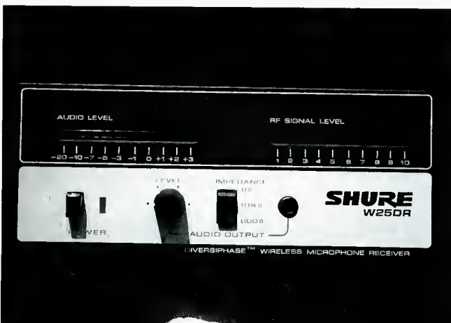
Figure 2. The front panel view of the W25DR Receiver.
