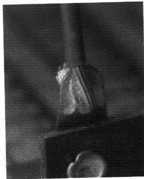
Fig. 7.8 Cold Solder Joint
