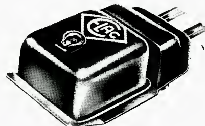
Fig. 4. Miratwin MST-1—a single unit available either for microgroove or standard records.
